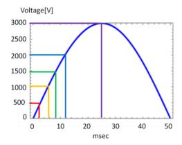
Figure 3: Required acceleration voltage per turn.
