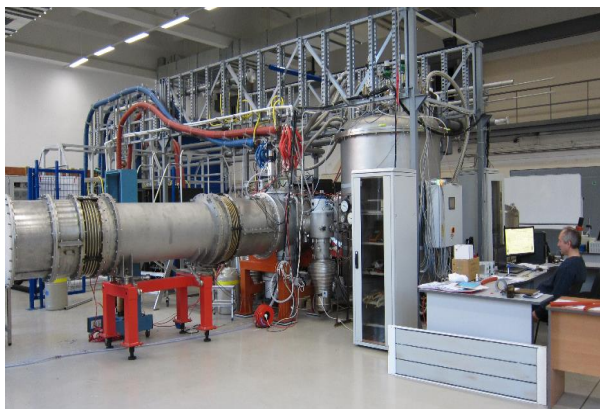
Figure 4: First bench of the SC magnet test facility.
