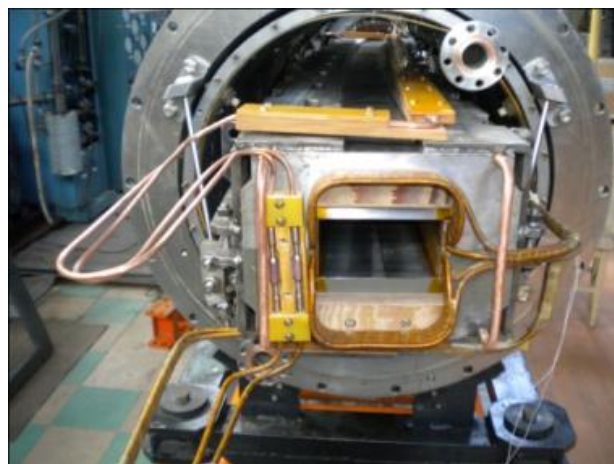
Figure 5: Pre-serial dipole magnet of the NICA Booster.
