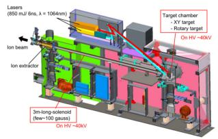
Figure 1: Cut view of the LIS.
