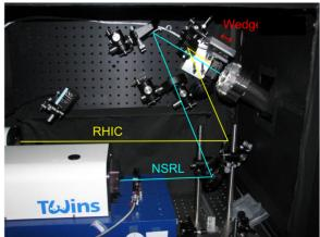
Figure 2: Laser paths in enclosure.
