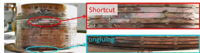
Figure 2: Internal injection helix defaults observed at 21 kA during the first test to reach 26 kA.
