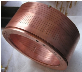
Figure 3: Perpendicular slits machined in the internal injection helix.
