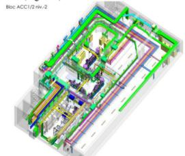
Figure 4: 3D views of processes + connections + buildings.
