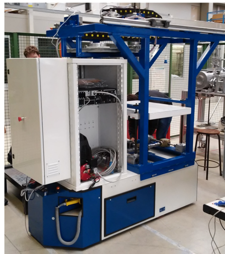
Figure 6: horizontal handling device made up of the AGV, the Cartesian system and the PLC control.
