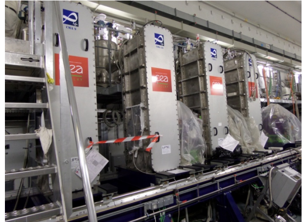
Figure 4: SPIRAL 2 RFQ installed in the linac tunnel.
