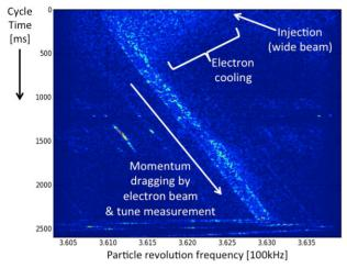
Figure 6: Schottky spectrum of the Ar<sup>11+</sup> beam as it is used for the new method of chromatic measurement.
