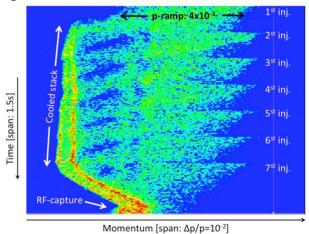
Figure 5: Schottky spectrum in momentum space of the Pb<sup>54+</sup> ion beam in LEIR in a waterfall diagram (time versus beam momentum).
