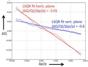
Figure 7: Measured machine tune deviation versus measured ion beam momentum deviation
