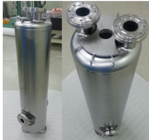
Figure 3: Quarter wave resonator after final electron beam welding.
