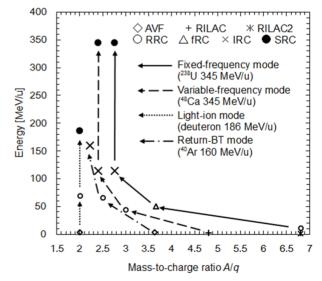
Figure 2: Transitions of energy and mass-to-charge ratio of accelerated nuclei in each acceleration mode in the RIBF.
