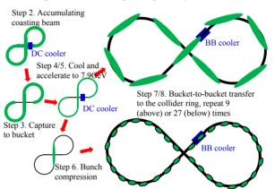
Figure 2: Illustration of the ion beam formation process, step 2-8 as listed above.
