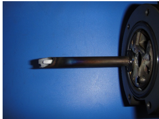
Figure 3: MgO rod with a stainless steel cover.
