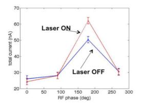
Figure 5: Measurements of 10 nA electron beam current using a lock-in amplifier.
