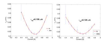
Figure 8: First thermal emittance measurement of  $Cs_2Te$  cathode.
