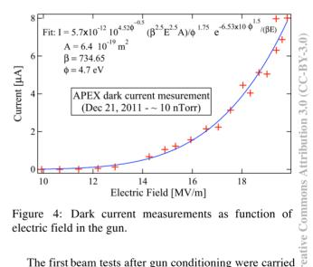
Figure 4: Dark current measurements as function of electric field in the gun.
