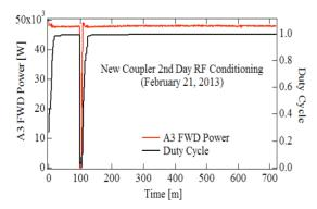
Figure 2: A 12-hour run at nominal power (50 kW each branch), showing no faults. The dip at 100 minutes was due to tunnel access.
