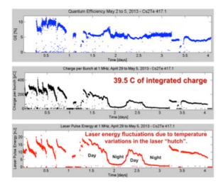
Figure 6: First measurement of cathode lifetime with MHz electron beam.
