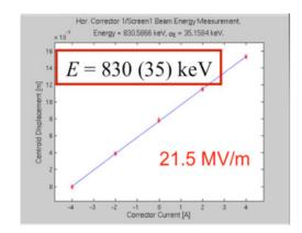
Figure 3: Electron beam energy measurement using a scanning coil.
