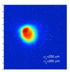
Figure 7: Transverse shape of laser pulse at the cathode for thermal emittance measurements.
