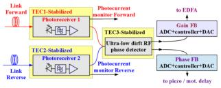
Figure 2: Block diagram of the low drift RF phase detector, used for stabilization of the pulsed BAM link.
