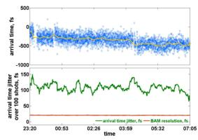
Figure 6: (upper plot) BAM drift measurement with the button pickup at mean charge 130 pC and with mean resolution 20 fs.
