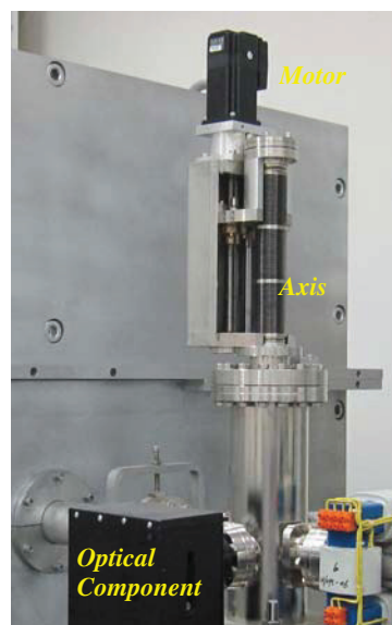
Figure 4: The assembled beam profile monitor.
