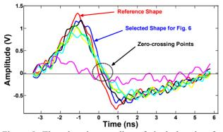
Figure 5: Time-domain recording of single bunches for different buncher amplitudes are depicted to determine the individual zero-crossing points.
