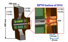
Figure 2: The technical layout of the inter-tank section.
