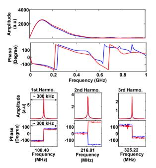
Figure 6: Amplitude and phase spectra for the reference shape (red) and the selected shape (blue) from Fig. 5. (up) from a single bunch, (down) from a stream of bunches (the amplitude spectrum nearly coincided).
