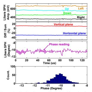
Figure 4: Single plate amplitude, position & phase reading within 1  $\mu$ s time resolution during one macropulse. The botton figure is the histrogram of the phase reading.
