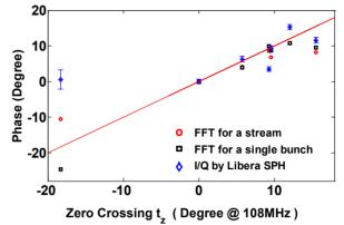
Figure 7: Time-domain data versus Libera SPH and FFT calculations for a single bunch and a stream of bunches.
