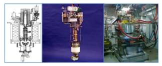
Figure 5: SLAC XL4 X-band klystron and assembly.
