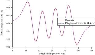
Figure 2: Field quality of an undulator with  $g = \lambda_u$ . Top left, vertical magnetic field  $B_{\nu}$  on centre plane of undulator. Top right, transverse map of  $B_{\nu}$  at longitudinal peak. Bottom,  $B_{\nu}$  along undulator axis (solid red line) and displaced by 5mm in H and V (dotted blue line).
