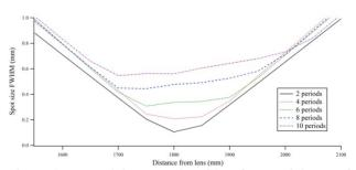
Figure 6: Focused beam waist of SR from undulators of different lengths. From ZEMAX simulation of a simple optical simple with 1:1 imaging.
