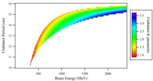
Figure 3: Undulator period and K parameter needed to produce 500 nm light at an opening angle of 2.5 mrad for different beam energies.
