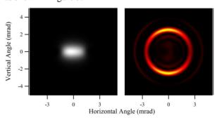
Figure 4: Total SR (left) and visible SR (right) from a 500 MeV electron beam crossing an undulator with 3 periods, K=1.3,  $\lambda_{u}=12$  cm. Simulated with SRW.
