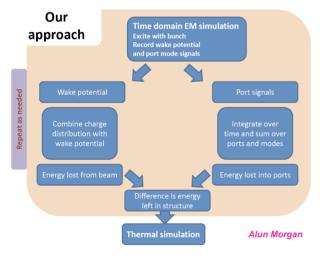
Figure 13: Approach being currently applied at the DLS to study the beam-induced RF heating [9].
