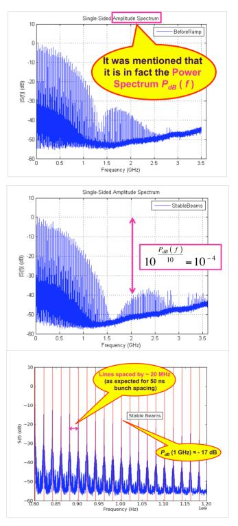
Figure 2: Power spectra measurements for LHC beam 1 on fill # 2261 (Courtesy of Themistoklis Mastoridis, Philippe Baudrenghien and Hugo Day).
