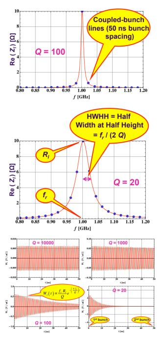
Figure 9: Impedance plots for a resonance with the resonance frequence  $f_r = 1$  GHz, shunt impedance  $R_l = 10 \ \Omega$ , for different values of quality factors Q and corresponding wake functions.
