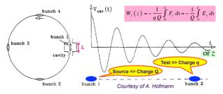
Figure 1: Illustration of the voltage induced by a bunch (bunch 1 in this example) going through a cavity. The bunch 2, at the distance z behind, will feel a longitudinal wake field given by the formula (more precisely, it is called wake function and it represents the response to a pulse of infinitely small length).
