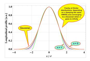
Figure 5: Family of (finite) distributions, keeping the same Half Width at Half Height (HWHH), depending on the parameter n, and converging to a Gaussian distribution when n goes to infinity.
