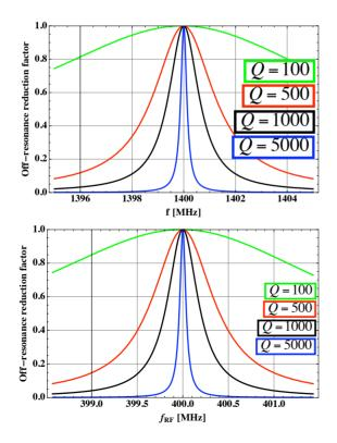
Figure 11: Off-resonance effect on the power loss, applied to the case of Fig. 10, vs. (a) the resonance frequency and (b) the RF frequency (assuming the resonance frequency at 1.4 GHz).
