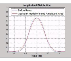
Figure 7: Longitudinal profile obtained by taking the inverse Fourier Transform of the measured spectrum before the ramp (see Fig. 2a; Courtesy of Themistoklis Mastoridis and Philippe Baudrenghien).
