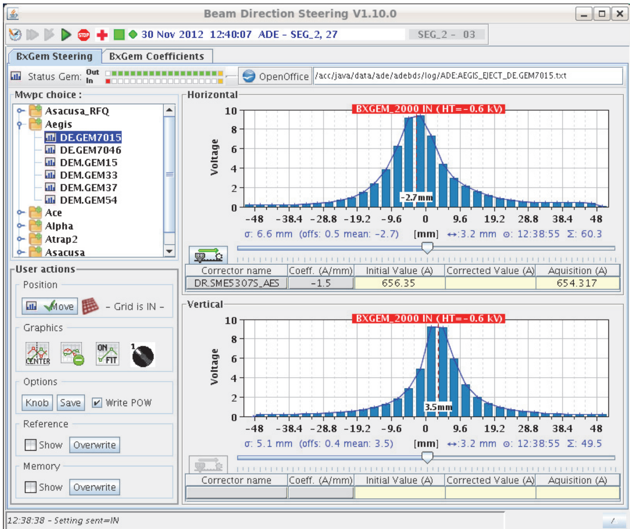
Figure 4: A screenshot from the graphical user interface from which the AD profile monitors are operated and read out.
