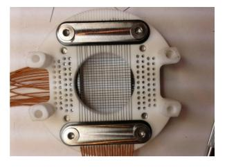
Figure 6: A photo of the ceramic piece holding the wires. The tiny threads for the grub screws are rather fragile and assembly using simple wire is difficult as wires start bending when the screws are fastened. The future design therefore uses the bands of a harp etched from a sheet of steel.
