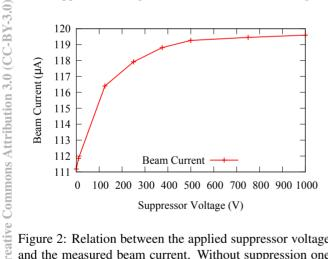
Figure 2: Relation between the applied suppressor voltage and the measured beam current. Without suppression one secondary electron for every ten  $H^-$  leaves the cup and falsifies the measurement. 500 V are sufficient to suppress most of this effect.
