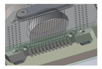
Figure 3: The Wire Grid with its ceramic assembly and grub screws for every single wire.
