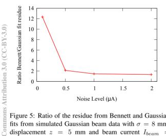
Figure 5: Ratio of the residue from Bennett and Gaussian fits from simulated Gaussian beam data with  $\sigma = 8$  mm, displacement z = 5 mm and beam current  $I_{beam} = 150 \ \mu$ A. At low noise levels it is easy to tell that the data comes from a Gaussian beam as the residue from the Bennett fit is far higher.
