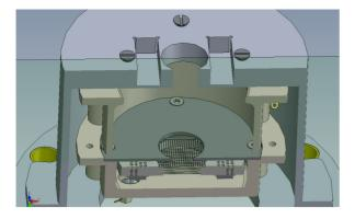
Figure 1: The Faraday Cup with the integrated Wire Grid.
