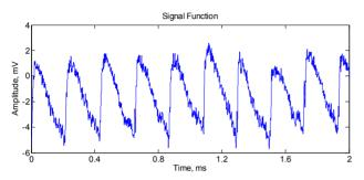
Figure 1: Example signal received from SM with a mirror as target.
