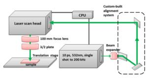
Figure 3: Ultra-short Laser configuration for materials processing.
