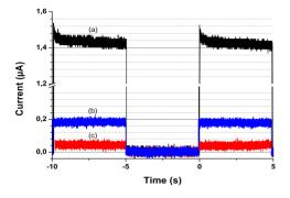
Figure 4: Full-bandwidth response of the FAIR-CCC to a rectangular current signal of 1.438  $\mu$ A (a), 185 nA (b), and 42.5 nA (c) applied to the additional calibrating loop.
