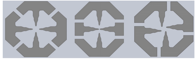
Figure 8: Different options for vane and body assembly.
