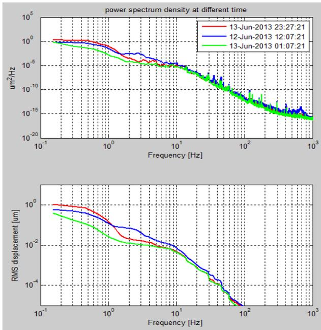
Figure 6: HXN satellite building floor vibration spectrum and cumulative RMS displacement at three different times.
