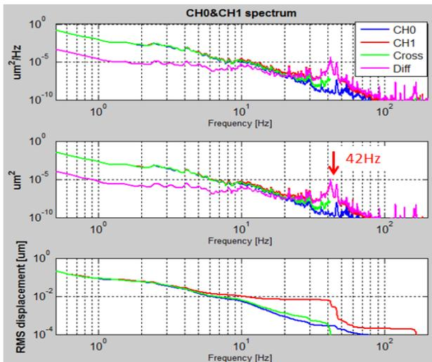
Figure 7: NSLS2 high stability BPM horizontal motion spectrum. Ch0- sensor sits on the floor; Ch1- sensor sits on top of the BPM stand.
