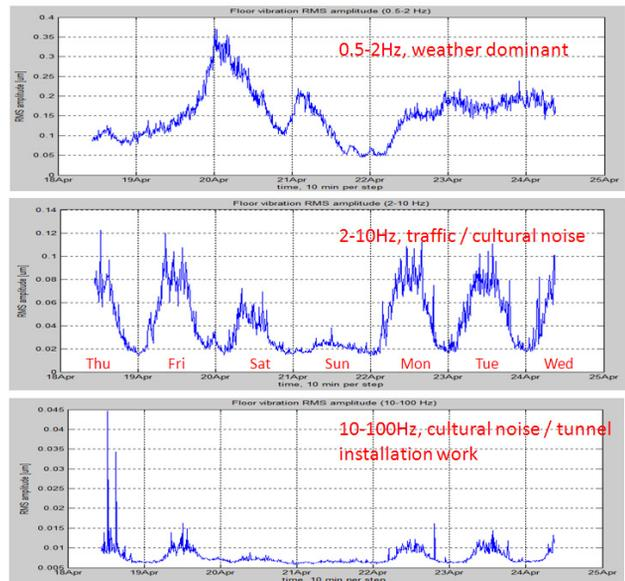
Figure 5: Integrated RMS motion in different frequency ranges for ~ 1 week period.
