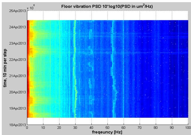
Figure 4: PSD spectrogram plot of NSLS2 tunnel floor motion during ~ 1 week period. Horizontal axis is frequency and vertical axis is the time at 10 minutes intervals. Color reflects the PSD spectrum amplitude.
