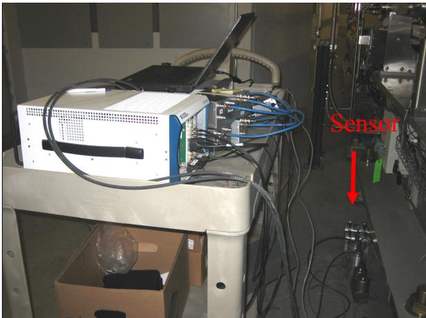
Figure 1: Vibration measurement setup in the NSLS2 storage ring tunnel.
