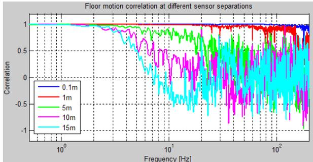
Figure 3: Two channel correlation at various sensor separations.
