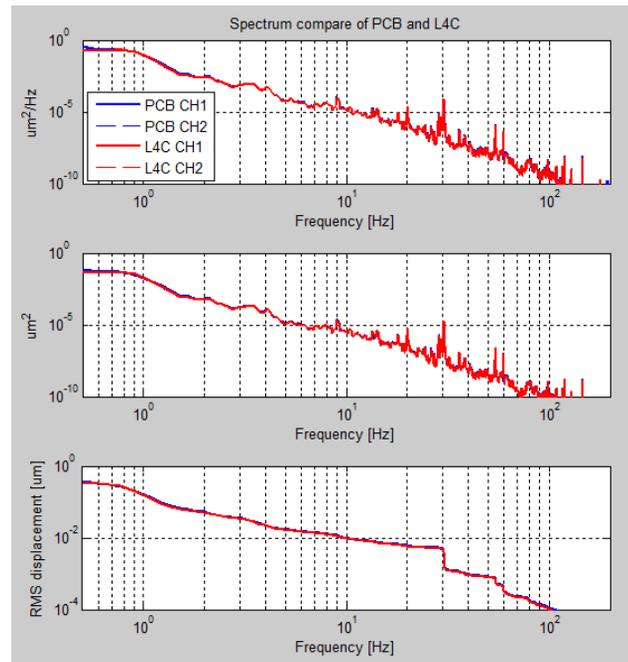
Figure 2: Typical ambient vibration spectrum measured on NSLS2 storage ring floor.
