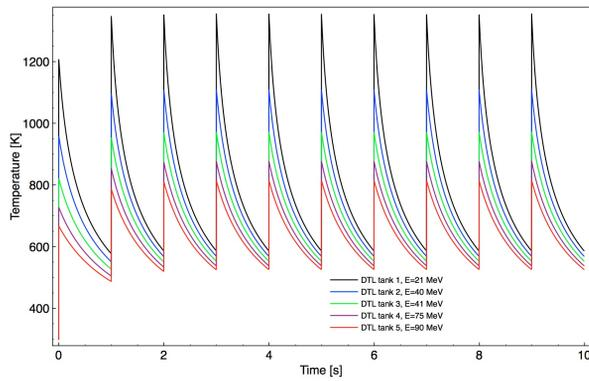
Figure 1: Maximum temperature on a carbon wire after each DTL tank (beam sizes are 1.5 mm in both planes).
