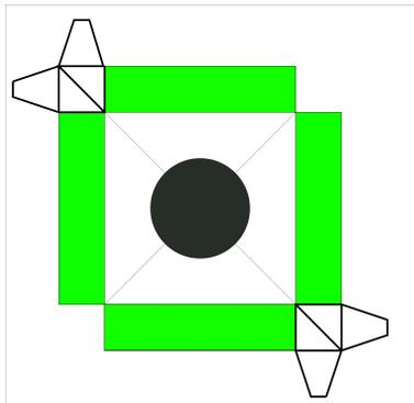
Figure 4: Scintillator geometry, in green the scintillator with the light guide (black line) and in grey the beam pipe.
