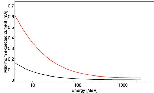
Figure 2: Maximum expected current on the wire in function of the beam energy, in red for a tungsten wire and in black for a carbon wire assuming  $\sigma_x = \sigma_y = 2\text{ mm}$ .
