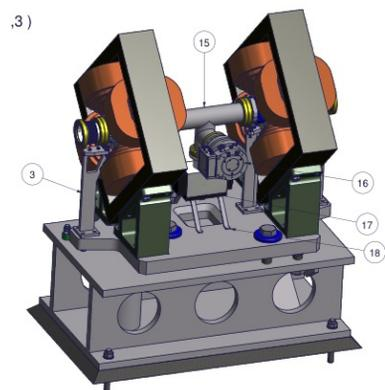
Figure 3: Warm Section Layout (courtesy of Aarhus University).
