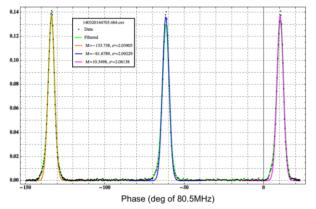
Figure 3: Typical bunch profile taken with phase shift technique. Peaks are distributed 72° apart.
