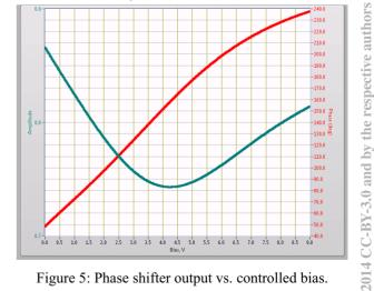
Figure 5: Phase shifter output vs. controlled bias.
