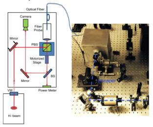
Figure 4: Laser transport line layout.
