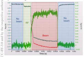
Figure 7: Macro-pulse structure during production. Red trace shows the MCP signal with laser hitting the ions and the grey-blue trace represents signal with laser being blocked by chopper. Green trace is the difference.
