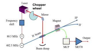
Figure 1: A layout of the Laser Bunch Shape Monitor.
