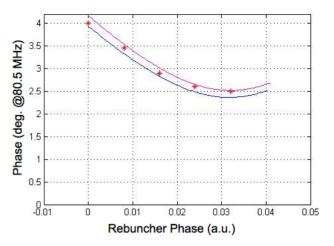
Figure 11: Experimental results compared to model generated for two different input Twiss parameters.
