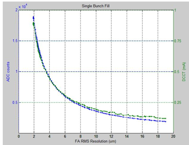
Figure 5: BPM FA data resolution with single bunch stored.
