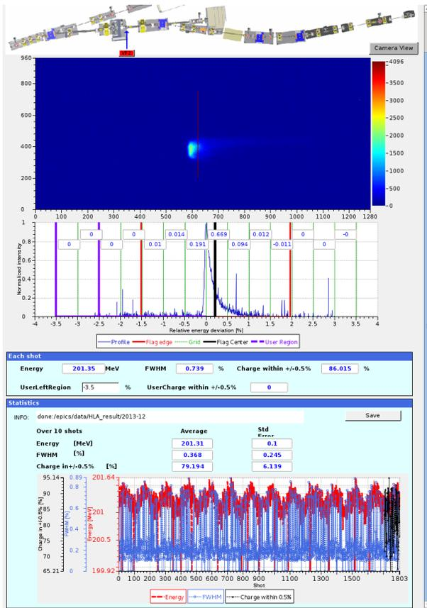
Figure 9: LINAC beam energy jitter and energy spread measurement using LtB VF2.
