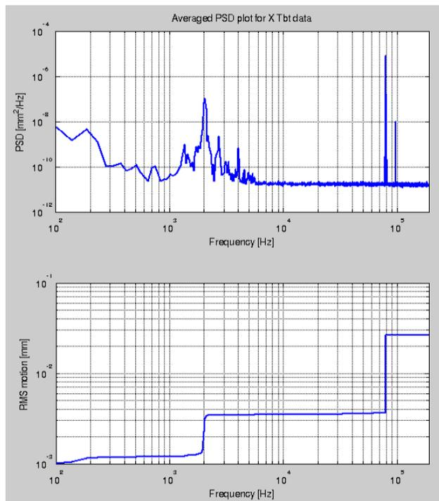
Figure 6: Averaged power spectrum density spectrum and integrated RMS motion plot from storage ring X TbT data. Beam was stored at  $23\text{mA}$ .
