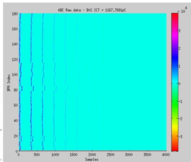
Figure 2: ADC waveform data from 180 SR BPMs, beam survived for about 5 turns. There are 310 ADC samples per turn.
