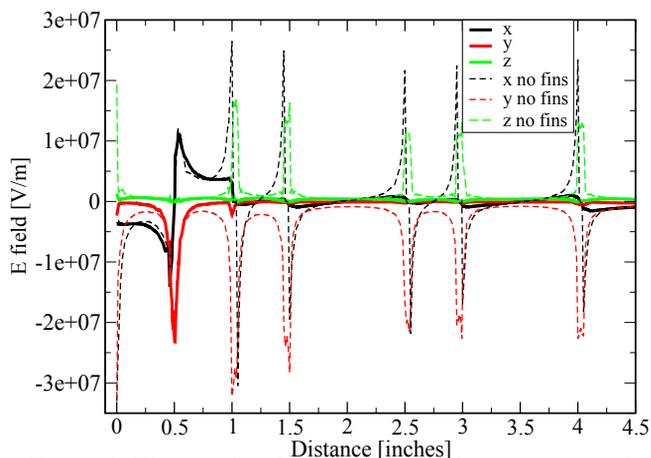
Figure 6: The simulated electric fields when target is in the center of beam (at 0.5 in location). Here z is along beam moving direction, y is the vertical direction and x is radial out direction. The solid lines are for the case with fins and the dashed lines are for the case without fins.
