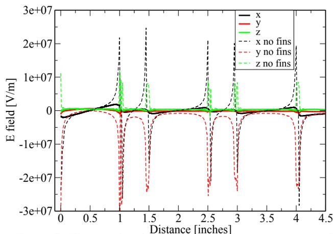
Figure 7: The simulated electric fields when target is out of beam. The coordinate system is the same as in Fig. 6.
