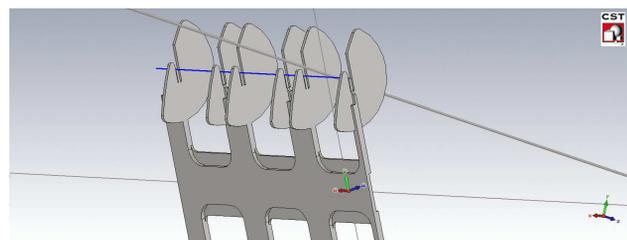
Figure 5: The details of the target frame fins. The shape is designed to have smooth curvature and enough clearance in the chamber. The half elliptical shape allows it to be mounted on every target, but a full elliptical shape should reduce the electric fields further.
