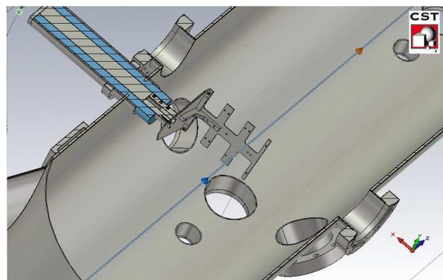
Figure 4: The detail of one horizontal target assembly. The vertical target assembly(the smaller hole at the bottom) was not included in the simulation.
