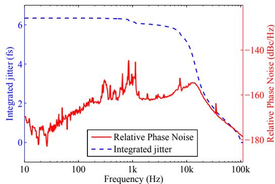
Figure 4: Phase noise data analysis of the TC780 laser locked to a TC1550 laser.
