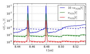
Figure 6: a[t] (solid) and  $r_m[t]$  (dashed) at the end of a 300 long 40 MHz pulse train.  $a_{ND0}[t]$  is offset by a factor 10 for readability.
