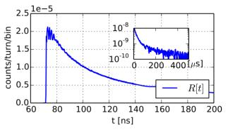
Figure 4: Single pulse afterpulse profile, R[t].
