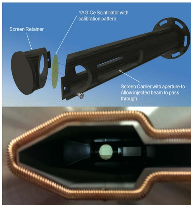
Figure 3: Screen carrier assembly and a beam's eye view of the YAG screen in the first turn position.
