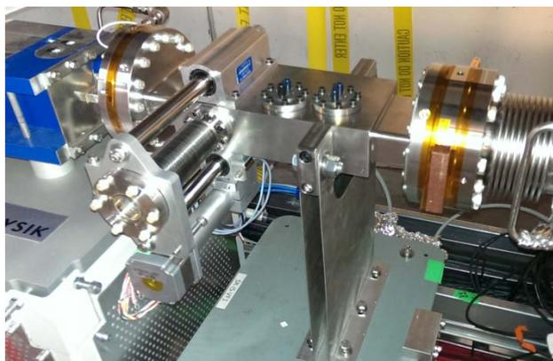
Figure 7: Installation of NSLS-II flag in the injection straight.
