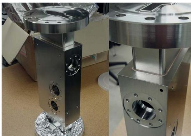
Figure 2: Successfully brazed flag chamber.
