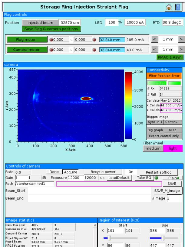
Figure 9: The interface control screen for the NSLS-II SR flag showing an image of the injected beam.
