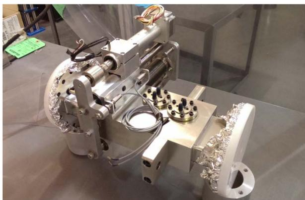
Figure 5: Final assembly of the NSLS-II SR Flag inside a portable clean hood.
