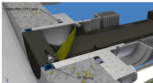
Figure 4: Screen in the parked position showing the RF spring. The HelicoFlex seal is also shown.
