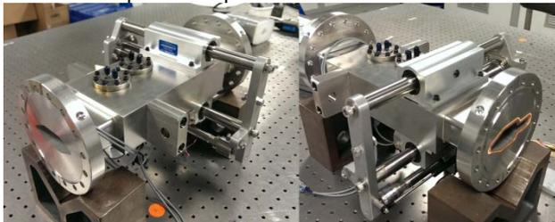
Figure 1: NSLS-II SR Flag in final assembly configuration.
