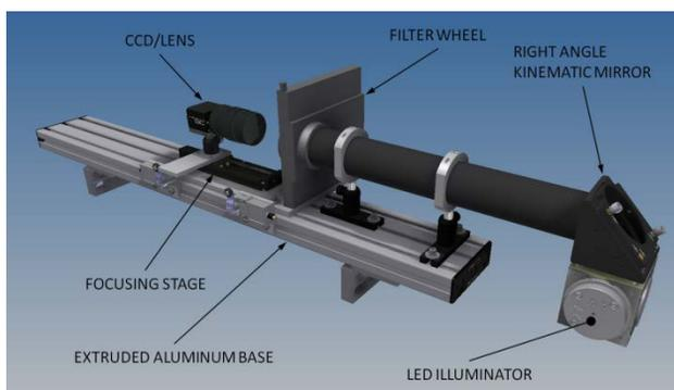
Figure 6: Details of the NSLS-II SR Flag optical transport.
