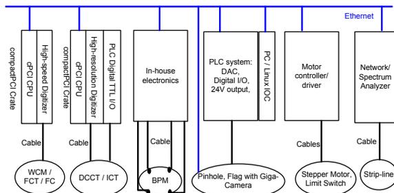
Figure 4: Diagnostics control interfaces.
