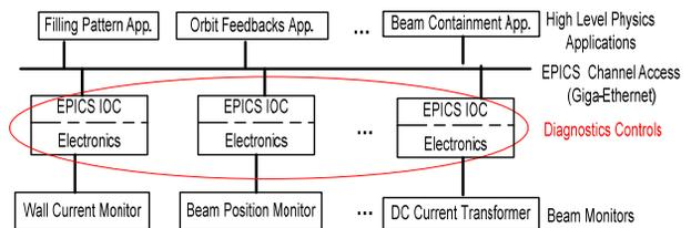
Figure 2: NSLS-II diagnostics and control architecture.
