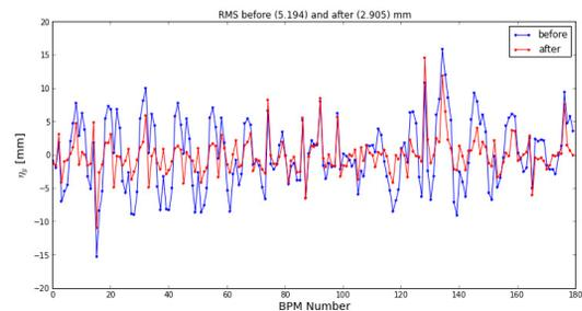
Figure 7: Preliminary test of slow orbit feedback.
