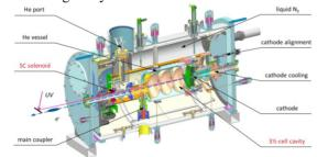
Figure 1: construction of the ELBE SRF Gun II.
