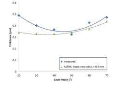
Figure 5: Transverse emittance versus laser phase.
