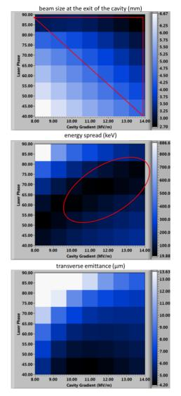
Figure 7: Simulation results: RF gradient and laser phase scanning for the beam with bunch charge of 1 nC. Results are given for the exit of the SRF cavity.
