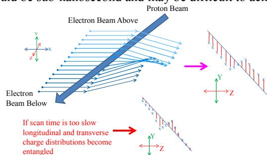
Figure 2: Fast scan of the electron beam though the proton beam. One can see the erf-like deflection from the baseline.
