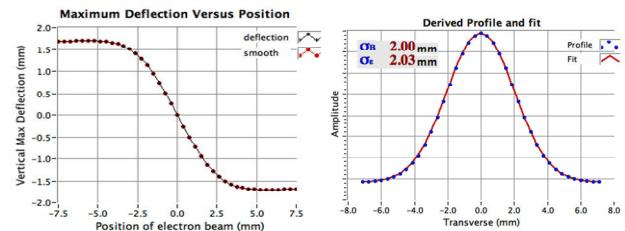
Figure 14: Deflection plot of electron beam, and the derivative of it, showing agreement to better than 2%.
