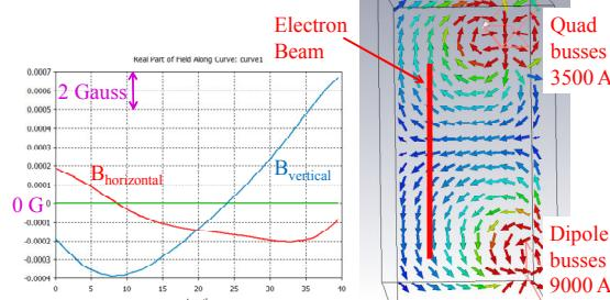
Figure 17: CST simulation of magnetic field from magnet busses along the line of the electron beam. The horizontal component is most important as the electron beam is vertical. The maximum horizontal field is 2 G.
