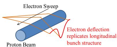
Figure 4: Deflection when the electron beam is scanned along the direction of the proton bunch with a duration equalling the bunch structure.
