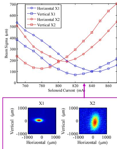
Figure 12: Horizontal and vertical rms beam sizes at the first (blue) and second (red) crosses in the test stand. The measurements are from OTR taken at  $\sim 50$  keV and 1 mA beam current onto the stainless steel mirrors.
