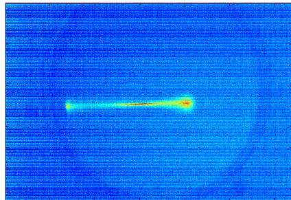
Figure 13: Trace of the electron beam on the phosphor screen for a deflecting voltage of  $\sim 150$  V. This image was not taken with the design optics. It was taken with just a camera and objective lens. The beam started off the screen on the left side and was then swept to the right.
