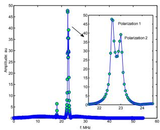
Figure 5: FFT of dipole waveform from Fig. 2. The sampling frequency is 108.3 MHz.
