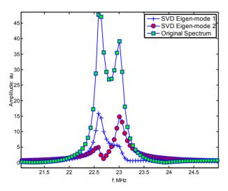
Figure 7: The identification of SVD modes and two polarizations of a dipole signal.
