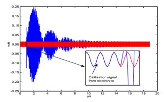
Figure 2: Dipole signal from HOM coupler 2 of 1<sup>st</sup> cavity at module 5. The calibration signal is highlighted with red colour and has a pure sinusoidal waveform.
