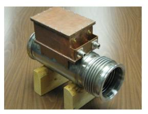
Figure 3: Short BPM detector (1).
