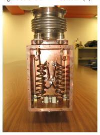
Figure 4: Short BPM detector (2).
