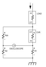
Figure 9: Measurement Equivalent Circuit.
