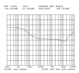
Figure 3: Apparent 1 m $\Omega$  CVR Frequency Response.
