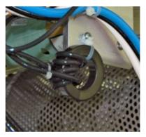
Figure 17: Multi-Turn Common-Mode Isolator.
