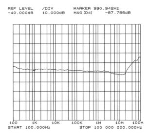
Figure 6: Improved 1 m $\Omega$  CVR Frequency Response.
