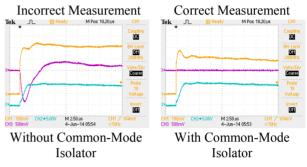
Figure 16: Example of Common-Mode Isolation.
