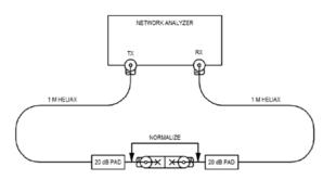
Figure 4: Cable-Current Artifact Measurement.
