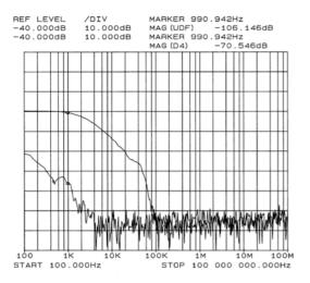
Figure 15: Performance of Common-Mode Isolator.
