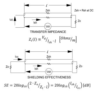
Figure 11: Cable Shielding Definitions [7]
