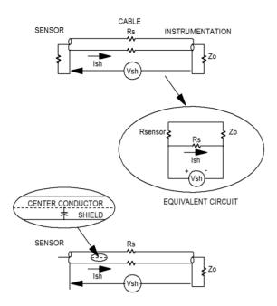
Figure 13: EMI Coupling into Shielded Cable.
