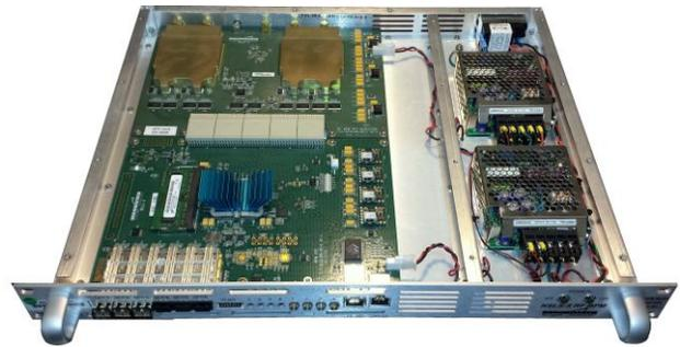
Figure 1: NLSL-II RF bpm electronics chassis.
