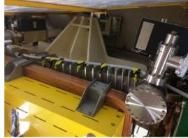
(a) Storage Ring scrapers (far left), Beam Loss Monitors be- (b) Optical f ber installed in the outer side of the bending maghind dipole (far right).
