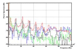
(b) Power spectrum for the 4 detectors (0, 100kHz)
