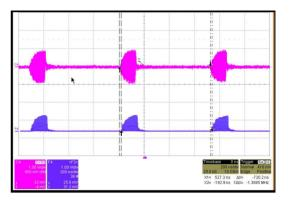
Figure 6: CLIC like pulse measured with the Fill pattern monitor
