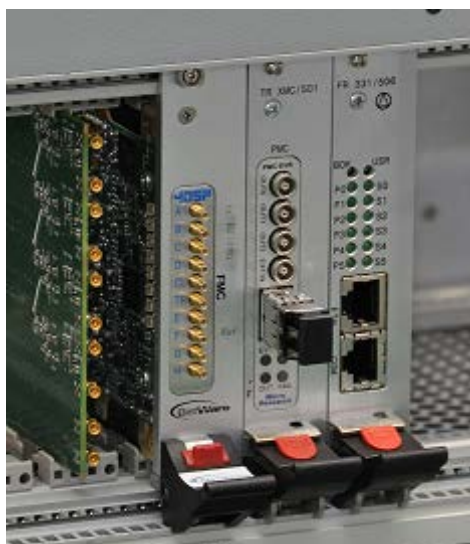
Figure 3: ASCU, FPGA, timing and network cards.
