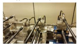
Figure 1: SwissFEL CBPM38 (left), CBPM8 with  $Q_L$ =1000 (middle) and CBPM8 with  $Q_L$ =200 (right).
