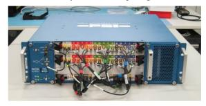
Figure 3: Cavity BPM electronics for two BPMs. Two RFFEs (top) and the FPGA carrier board with ADC mezzanines (bottom) are inserted into a customized crate from the front side. Power supply module and boards with SFP+ transceivers etc. are plugged in from the rear side.
