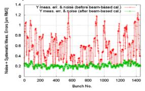
Figure 6: Floating average of the Y RMS measurement error (noise plus systematic errors due to switching attenuators etc). of FLASH CBPMs vs. bunch number before and after beam-based calibration of attenuators, calculated by correlating the readings of three CBPM10.
