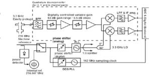
Figure 2: Simplified schematics of low-Q CBPM RFFE electronics, showing only one of its three input channels.
