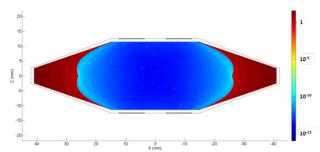
Figure 4: Error between the theoretical beam position and the rebuild position using boundary element and Newton inversion method with the additional lob correction. In the area of interest ( $\pm 15$ mm in H,  $\pm 10$  mm in V around the BPM centre), the error is below 10<sup>-10</sup> mm
