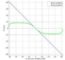
Figure 2: Read beam position (green) with respect to the real beam position (blue) in the horizontal plane for a centred beam in vertical plane. Linear region is limited to  $\pm$  2mm around the BPM centre.
