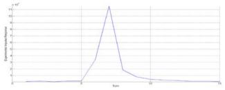
Figure 8: Impulse response of the BPMs measured when the beam is doing only one turn in the storage ring. Electronics filters over  $\sim 6$  turns to produce turn-by-turn samples.
