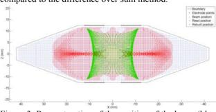
Figure 3: Reconstruction of the position of the beam (blue points) using the difference over sum method (green points) and the Newton inversion (red points).
