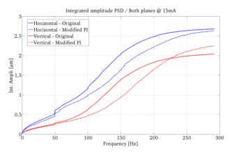
Figure 14: Integrated spectrum improvement when using the modified PI regulator for the correctors power supplies on a 15 mA beam.
