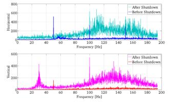
Figure 8: FFT spectrum comparison before and after the shutdown when running the FOFB @ 15 mA beam.
