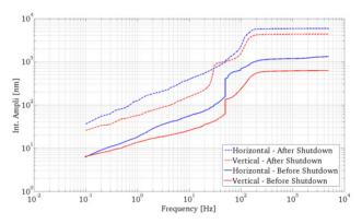
Figure 9: Integrated spectrum comparison before and after the shutdown when running the FOFB (a) 15 mA beam.
