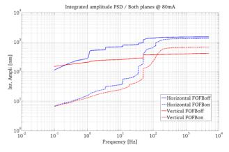
Figure 4: Integrated spectrum of both planes, with FOFB running or not. Beam is excited at different frequencies using a trim coil power supply.
