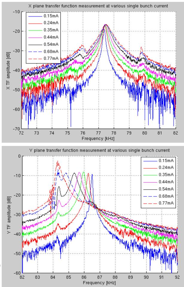
Figure 3: Single bunch transfer function measurement at various bunch current for horizontal (top) and vertical (bottom) plane.
