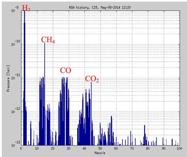
Figure 8: Typical residual gas analyzer (RGA) measured results with beam stored in the ring.
