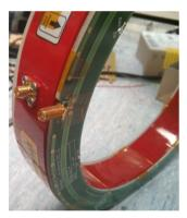
Figure 7: The installed calibration winding.
