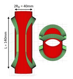
Figure 2: Example for the winding of one wire for Scanner coil (green) on the beam pipe (red).
