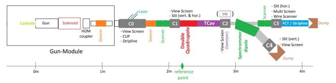
Figure 1: Schematic view of GunLab.
