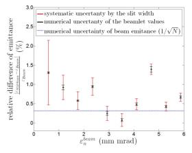
Figure 4: Relative differences between beam emittances and measured emittances by slit scanner.
