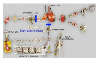
Figure 3: Composite photo of the ANU LINAC facility; the locations of the beam pulse monitor systems are marked in blue colour.
