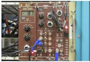
Figure 2: The electronic modules used by the beam pulse monitor system. From left to right: high voltage supply for the BaF2 detector (Ortec 556), time-to-analog converter (Ortec 567) and constant fraction discriminator (Ortec 584). The Single Channel Analyser in the TAC module is not used. The modules are installed in an Ortec 4001C NIM bin.
