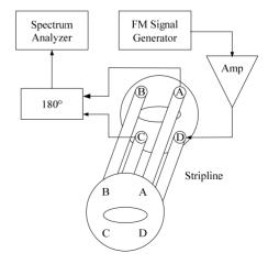
Figure 3: Layout of the tune measurement system at the SPS storage ring.
