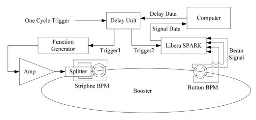
Figure 1: Layout of the tune measurement system at the SPS booster.
