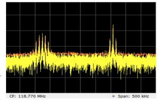
Figure 5: Result of tune measurement using FM signal. Peaks on the left are for vertical tune while peaks on the right are for horizontal tune.
