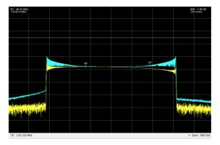
Figure 4: FM signal on spectroscope in real-time mode (yellow) and max hold mode (blue). The center frequency is 118.79 MHz with 500 kHz span.
