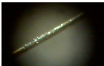
Figure 5: Gold coating melted off wires used at IP for 20 by 20 beams.
